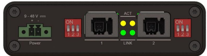
Illustration 3: Interface for power, DIP switches for link configuration and 100/1000BASE-T1 interfaces
