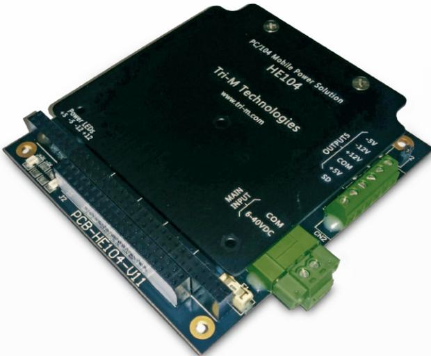
The HE104 is a high efficiency, high performance DC to DC 60 watt converter with an ultra-wide input range of 6-40V and supplies 5V, 12V and optionally -5V and -12V. The HE104 is specifically designed for rugged and hostile vehicular applications. The three stage input protection circuit includes an input filter, 10,000W heavy duty transient suppressors and an active Mosfet and controller surge stopper. The HE104 has an opto-coupled 6 to 40V input for remote On/Off control.
