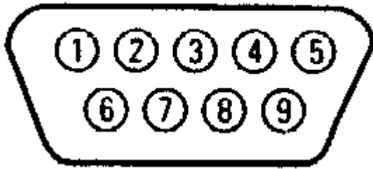
Figure 6: ECR – RS232 interface connection
