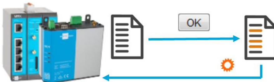
Figure 9: Profile handling – activating configuration modifications
